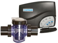
The **AquaRite® 100** is easy to install in existing pools and produces up to 20% more chlorine than other similar systems on the market. The unit operates at flow rates as low as 20-25 GPM and over a wide salt range: 1500 and 4500 PPM.
