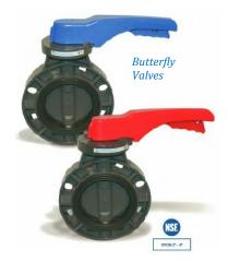
Butterfly Valves are constructed with a one piece body that incorporates fully supported flanged bolt holes to prevent stressing of the mating pipe flanges. Features include PVC bodies and discs, EPDM liners and seals and a SS316 shaft. Valves are rated to 150 psi
