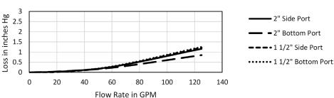
Head Loss Curves WG1048E on Sump
